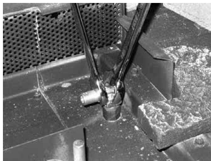
Burner Orifice Removal
