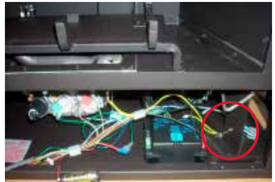
The Surefire switch is located in the right corner of the bottom louver/panel.
