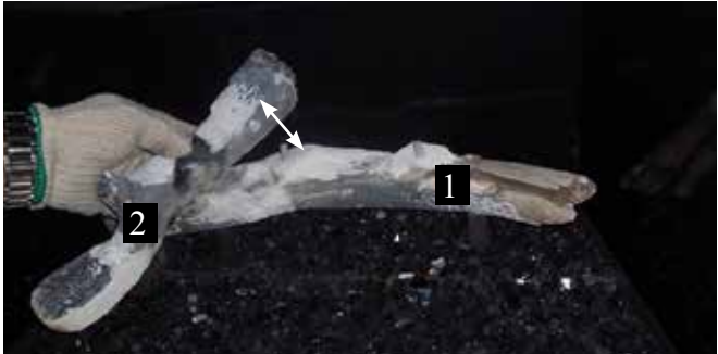
Log 2 pin locator match with Log 1 pin
