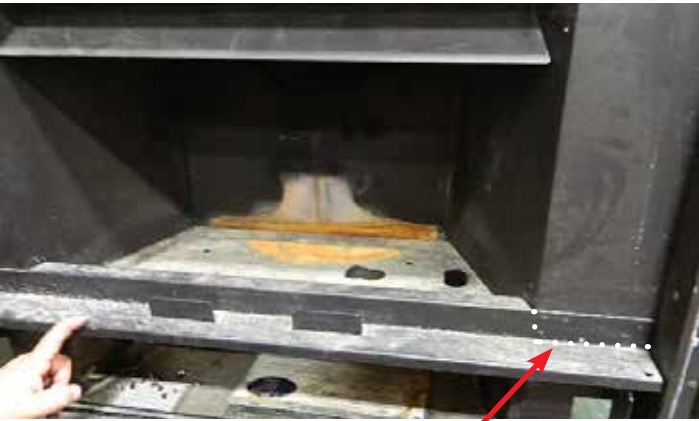
Diagram 6 Cut here to remove bar
