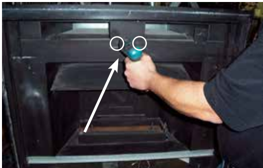
Remove 2 screws - remove Top Bracket
