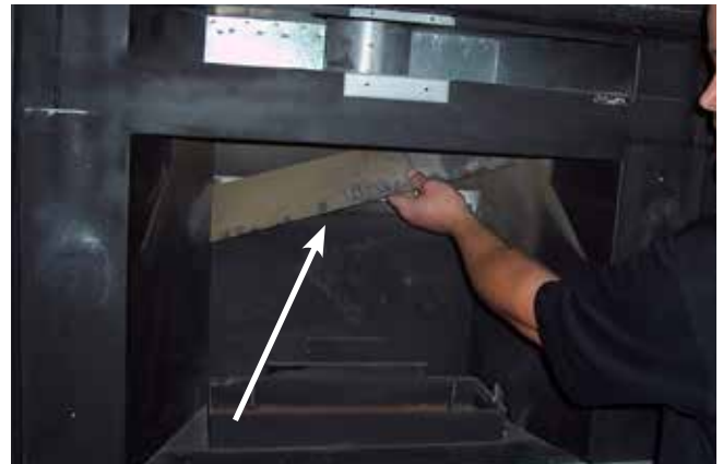
Remove rear baffle
