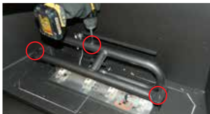
Diagram 2: Slide burner assembly to the right—then remove.
