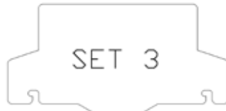
Restrictor plate for Set 3 (Part # 761-143F)
