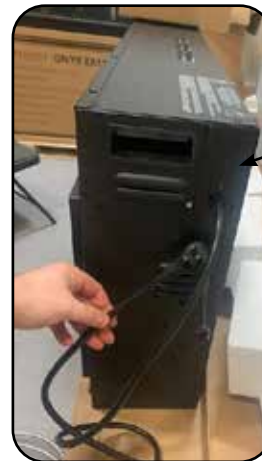
Wire Harness & Cover Plate Reinstalled.
