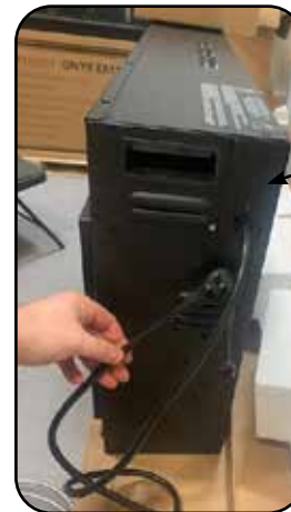
Wire Harness & Cover Plate Reinstalled.
